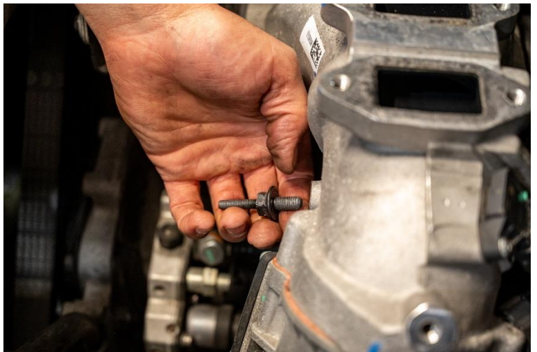
Figure 28: Removal of threaded stud on factory intake horn.
