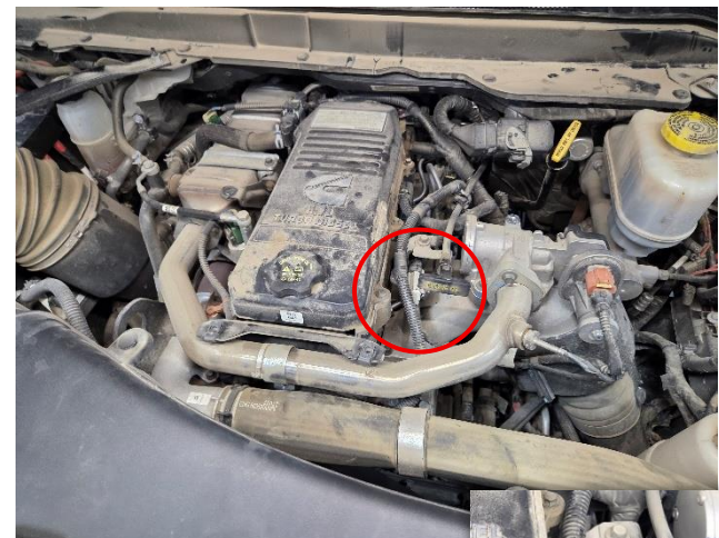
Figure 8: EGR temperature sensor connector on cab and chassis models, circled for clarity.
