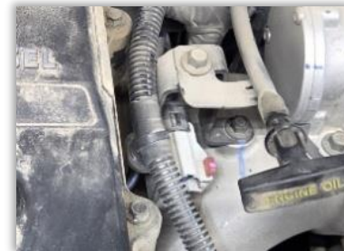
Figure 48: Example image of EGR crossover tube temperature sensor reinstalled.
