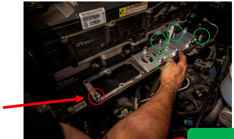
Figure 21: Intake plenum installed, M8 1.25x25 bolts circled.
