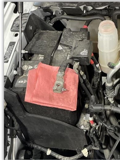
Figure 4: Use of shop towel to isolate negative terminal.
