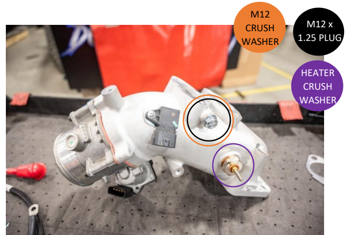
Figure 31: M12 plug and washer installed. New heater and crush washer installed.
