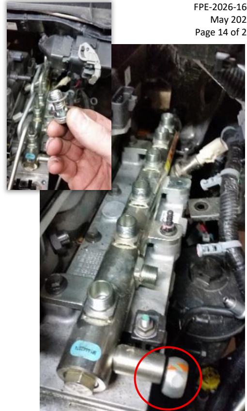
Figure 16: Injection lines removed, fuel return line circled.
