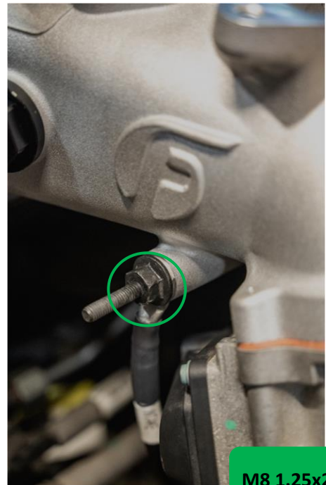
Figure 41: Heater ground cable installed at intake horn.
