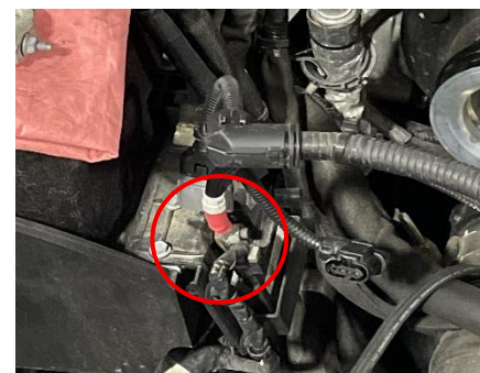
Figure 13B: 13MM nut retaining grid heater power supply harness.
