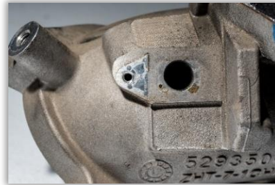
Figure 8A: MAP sensor location on intake horn.
