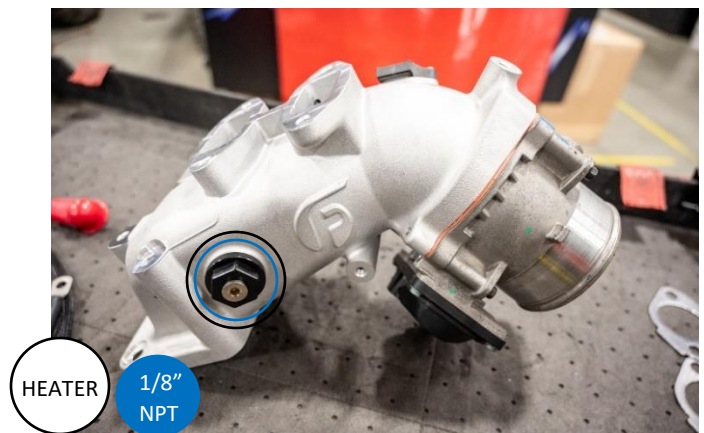
Figure 32: Heater plug and 1/8" NPT installed.
