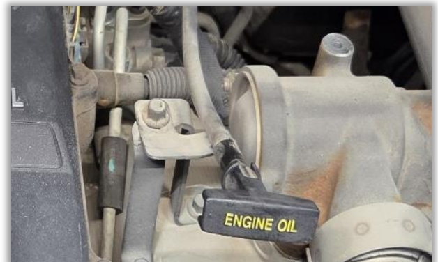
Figure 6: three 10MM bolts and bracket retaining oil dipstick tube.
