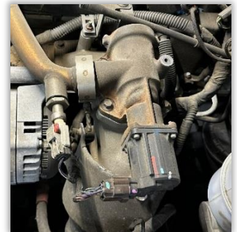
Figure 47: Example image of EGR Valve electrical connector and crossover tube temperature sensor, reinstalled.
